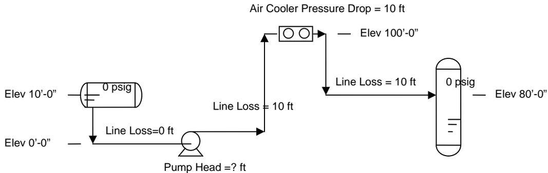
In order for the flow to occur according to direction of the arrow heads and for the system to stay away from vacuum,
